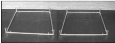
1. Assemble two squares using 4 unwedged pipes and 4 corner fittings for each.
