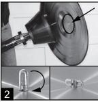
Attach unit through the reflector center hole. Flip the folding wing nut and screw down onto reflector until secure
