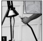
Snap legs in place. Attach base stabilizer for added stability.
